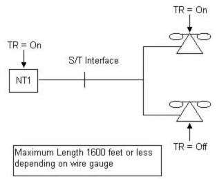
Fig. 7: Terminating Resistor Settings for Equal Distance Telesets
